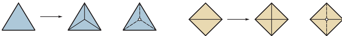
FIGURE 3.1. Two types of stellar subdivisions in the plane. The circle and dashed lines indicate the added vertices and edges.
